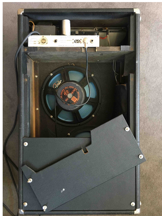
Fig. 3: a) left: the angled front panel arrangement with cooling slits. Could they have pointed out any more strongly that transistors were at the heart of this amp ... b) right: with the upper rear cover panel removed, the modular arrangement of power-amp/supply and preamp becomes visible. At some point, the original fender speaker plug was replaced by a larger plug necessitating the small cutout in the cover.
