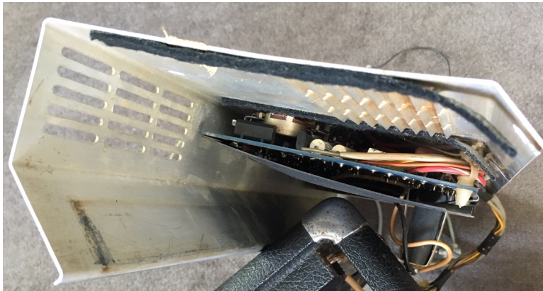
Fig. 8: Side view of the removed preamp module - the edge on the lower left sits in a groove in the lower panel of the amplifier compartment.
