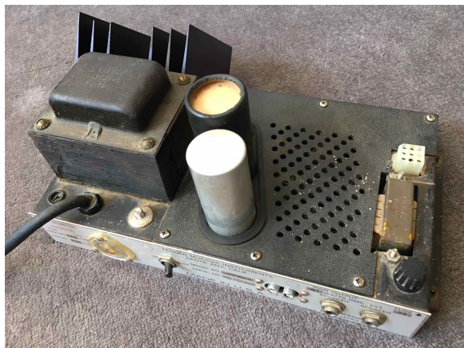
Fig. 5: power module from the top. Note the special, custom made rubber "gasket" surrounding the capacitors to avoid extra mechanical loading on components and printed circuit board.
