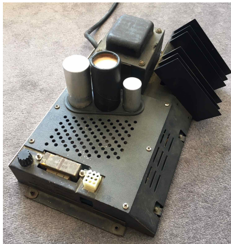
Fig. 5: power module from the top. Note the special, custom made rubber "gasket" surrounding the capacitors to avoid extra mechanical loading on components and printed circuit board.
