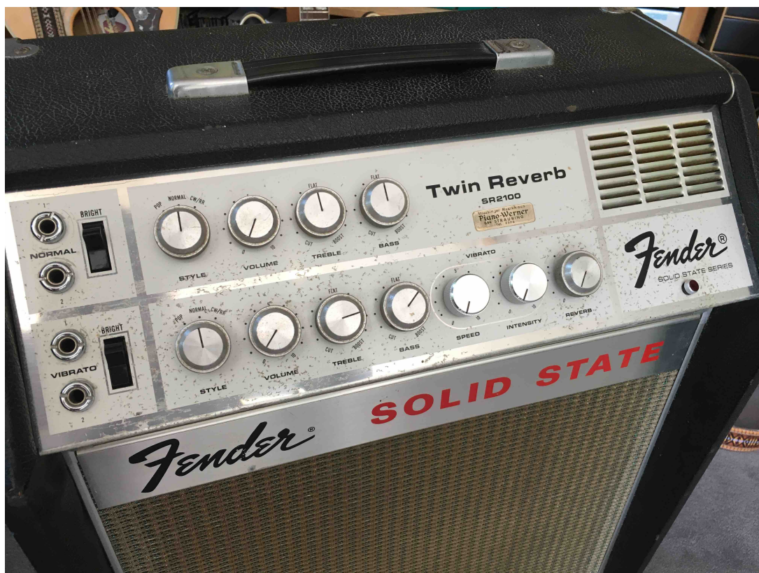
Fig. 2: The control panel up-close. The controls on the left are the "style-switches": Pop-Normal-RR/CW. The tremolo-control knobs are not original, and the little label below the designation is the sticker of the shop (in a small provincial town in the south east of Germany) that sold the amp. (N.B.: that shop still does business - not a bad feat, either!).
