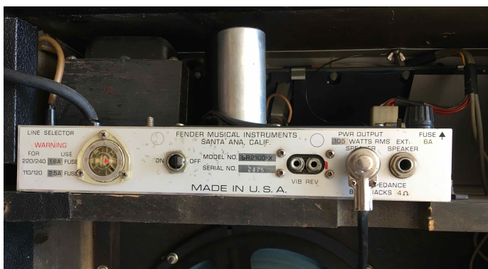
Fig. 4: view of the power module from the rear. It features (from left to right): a voltage selector (it is an export model, after all) with included fuse holder, a single on/off-switch (solid-state!), the input and output jacks to connect the reverb spring, the regular speaker jack, and the jack for an extension speaker. Above the upper right-hand corner sits a fuse-holder for the fuse incorporated in the speaker output.
