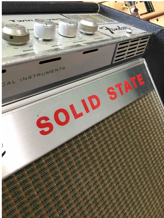
Fig. 3: a) left: the angled front panel arrangement with cooling slits. Could they have pointed out any more strongly that transistors were at the heart of this amp ... b) right: with the upper rear cover panel removed, the modular arrangement of power-amp/supply and preamp becomes visible. At some point, the original fender speaker plug was replaced by a larger plug necessitating the small cutout in the cover.
