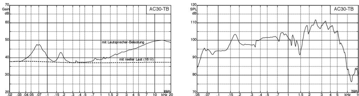
**Fig. 10.10.32 left:** VOX AC30-TB, transmission from phase-inverter-input to loudspeaker-output; dashed: with resistor; solid: with speaker; **right:** transmission from Normal-input to SPL in the AEC, volume = 12:00 h.
