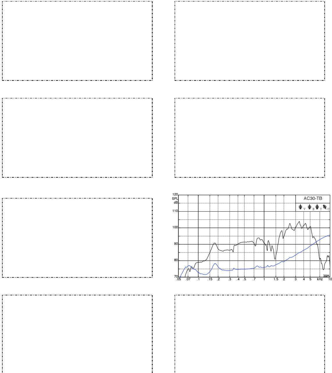
**Fig. 10.10.34:** SPL ( $d = 2\text{m}$ ) and voltage level (lower curve).
